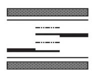
heating plate top teflon glass fabric structured Elastosil E43 N<sup>2</sup>) conveyor belt (conveying site up) Elastosil E47 1) conveyor belt (conveying site up) teflon glass fabric structured heating plate bottom
