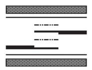
heating plate top teflon glass fabric structured Elastosil E43 N<sup>2</sup>) conveyor belt (conveying site up) Elastosil E47 1) conveyor belt (conveying site up) teflon glass fabric structured heating plate bottom
